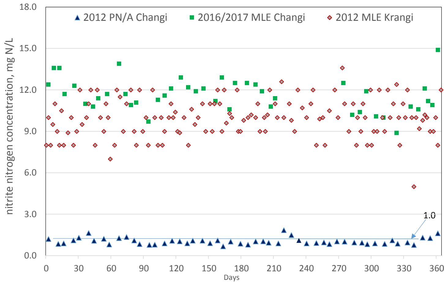
Almost 10 mg NO<sub>3</sub>-N/L less than conventional BNR process!
