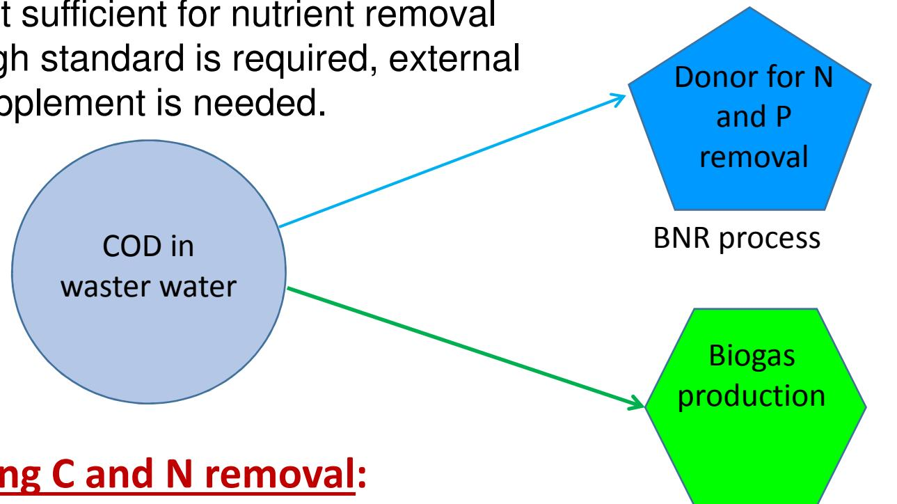
**Decoupling C and N removal:**
